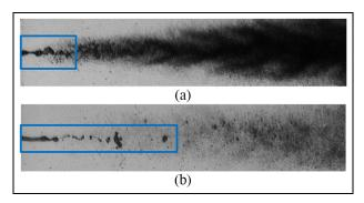
**Figure 11.** Raw DBI images obtained at (a) 160  $\mu$ s and (b) 2.4 ms after the closure of the injector needle. Dribbling fuel is highlighted by the blue rectangles. Top and bottom images correspond to following experimental conditions:  $P_{\rm inj} = 500$  bar,  $P_{\rm g} = 26$  bar and  $T_{\rm g} = 293$  K.
