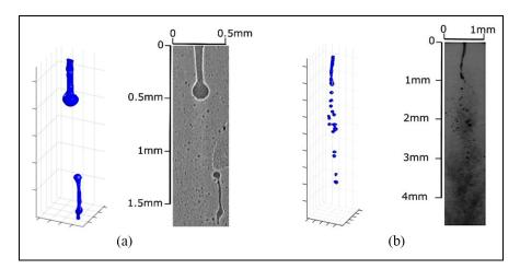
**Figure 4.** Raw images with results of 3D reconstruction, from (a) X-ray phase-contrast technique ( $P_{\rm inj}$  = 500 bar;  $P_g$  = 30 bar;  $T_g$  = 297 K) and (b) DBI image ( $P_{\rm inj}$  = 500 bar;  $P_g$  = 27 bar;  $T_g$  = 293 K). Images (a) and (b) were captured after 132.6  $\mu$ s and 333  $\mu$ s after the end of injection.
