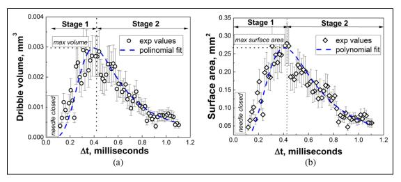
**Figure 6.** Dribble volume (left image) and surface area (right image) versus time. Both diagrams obtained by processing of X-ray images which correspond to the following conditions:  $P_{inj} = 1000$  bar,  $T_g = 297$  K and  $P_g = 30$  bar.
