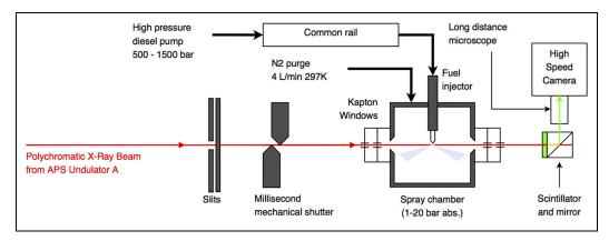
Figure 2. Schematic diagram of the X-ray phase-contrast imaging experiments. The diagram is not to scale.
