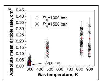
**Figure 12.** Dependence of the absolute mean dribble rate on the gas temperature  $T_g$ . Argonne data are highlighted by the blue rectangle. Averaged values of the absolute mean dribble rate are shown by red symbols.
