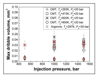
**Figure 9.** Dependence of maximum dribble volume on injection pressure  $P_{\text{inj}}$ . Averaged values of the maximum dribble volume are shown by red symbols.
