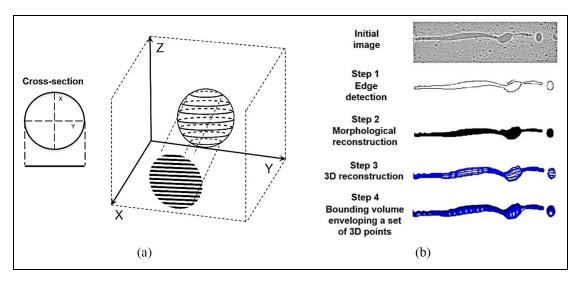
Figure 3. (a) Schematic of the object model and (b) main steps of the image processing algorithm. X-ray phase-contrast image was used to show different steps of image processing (see initial image).
