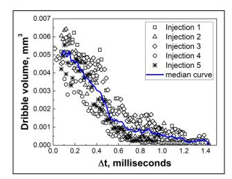
**Figure 7.** Time dependence of dribble volumes obtained from Argonne data for the following experimental conditions:  $P_{\rm inj}$  = 500 bar,  $T_{\rm g}$  = 297 K,  $P_{\rm g}$  = 30 bar and  $\rho_{\rm g}$  = 34 kg/m³. Obtained dribble volumes correspond to a sequence of injections which were obtained at similar experimental conditions.
