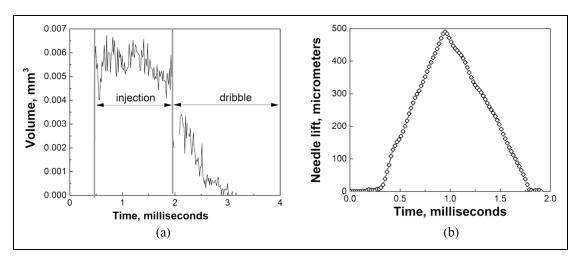
**Figure 5.** Time dependence of the liquid volume during the injection process for:  $P_{inj} = 1500$  bar,  $T_g = 297$  K and  $P_g = 20$  bar. (a) Experimental data and (b) needle lift values are provided by Argonne.
