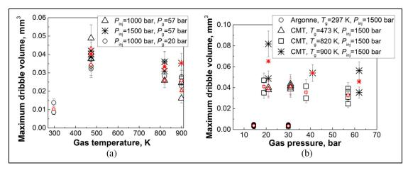
**Figure 10.** Dependence of the maximum dribble volume on (a) gas temperature  $T_g$  and (b) gas pressure  $P_g$ . Averaged values of the maximum dribble volume are shown by red symbols.
